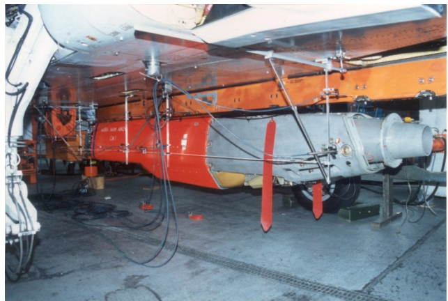
Figure 35: Stiffness Test under fuselage Store.
