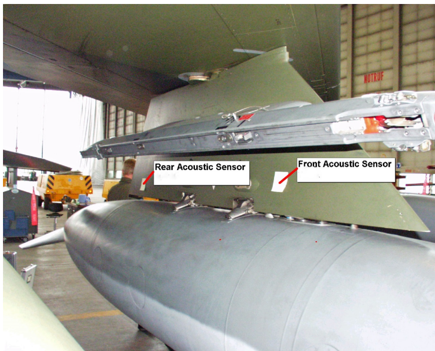
Figure 39: Location of Acoustic Sensors on Tornado I/B Pylon with Tank and Stub Pylon.
